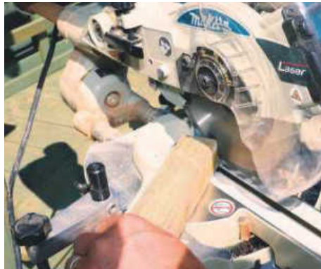
STEP 5. Use the shoulder line as the gauge and make a second cut, then rotate and repeat
